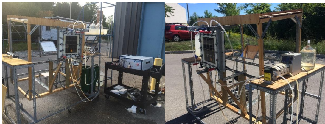
Figure 27 The experiments under concentrated sun light for photoelectrochemical hydrogen production integrated to ammonia synthesis
