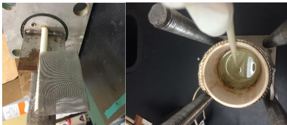
Figure 7 Nickel mesh electrodes in the reactor, molten salt in the reactor
