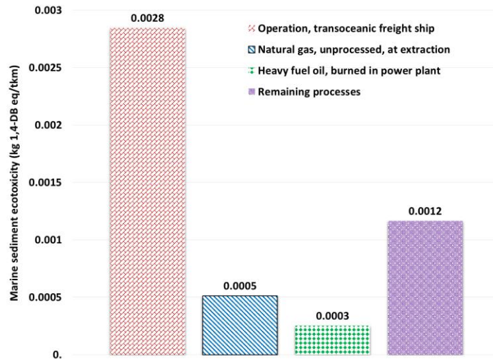
Figure 60 Process contributions to marine sediment ecotoxicity values of transoceanic freight ship fueled by sole ammonia from municipal waste
